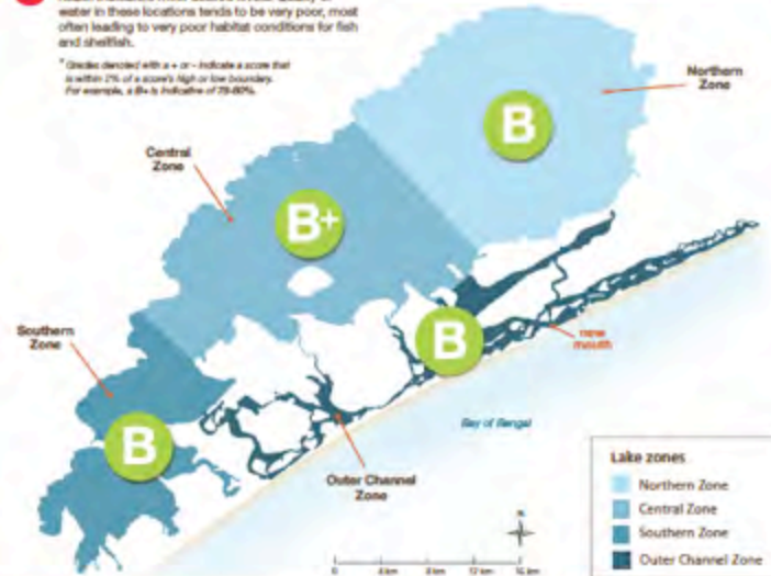
Until recently, Chilika Lake suffered from increasing sediment loads and reduced connectivity with the sea. In 2002, a new mouth to the Bay of Bengal was opened. This hydrological intervention helped improve salinity levels, enhance fish landings, decrease the size of invasive species, as well as improve water quality overall.
