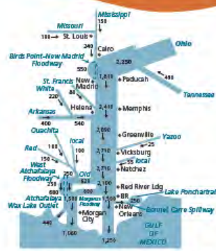
Flow capacity for the Mississippi River in thousands of cubic feet per second, based on the 1956 project design flood. Graphic courtesy US Army Corps of Engineers.
