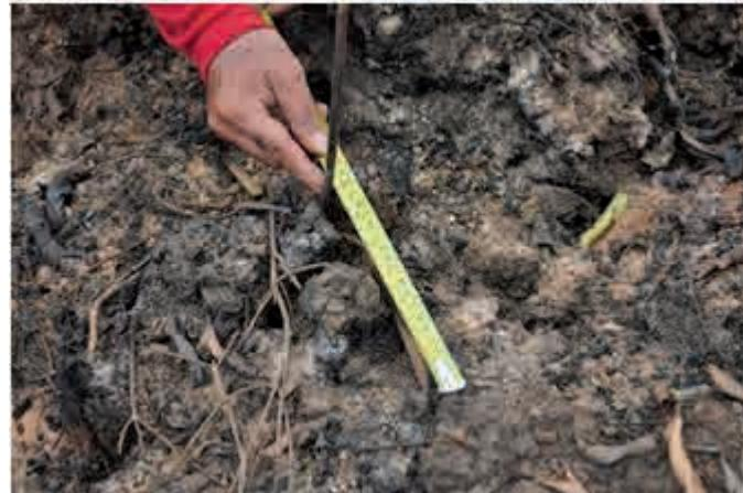
Figure 25: Metal tape measure measuring horizontal distance from metal rod to the closest edge of where the peat. Note the etch mark on the rod used for measuring the depth to where the peat burned
