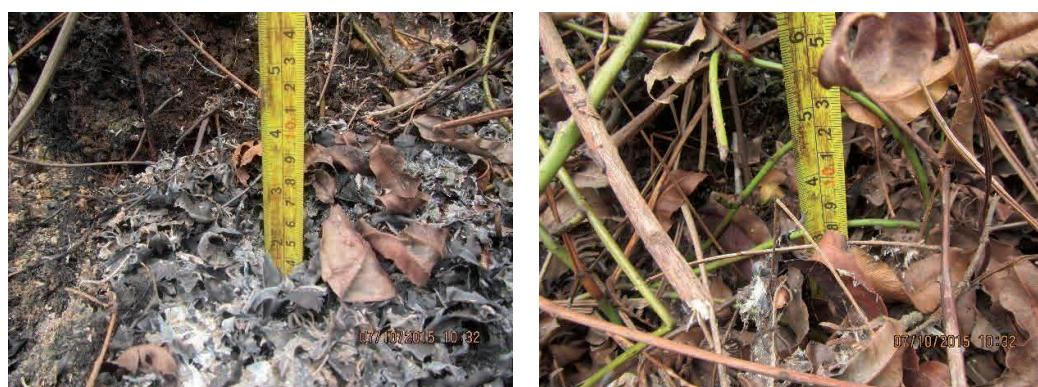
Figure 6: Tape measure used to measure top of surface fuel to top of the peat layer, both after and before the burn
