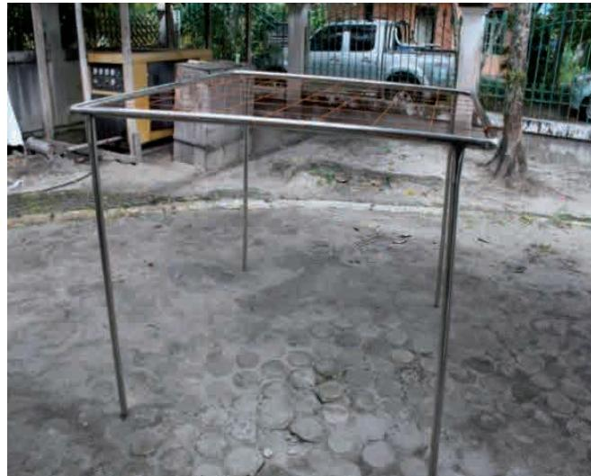
Figure 29: Stainless steel frame for taking the peat volume loss measurements
