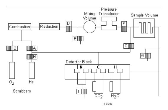
Schematic diagram of the Exeter Analytical, Inc. (EAI) CE-440 Elemental Analyzer
