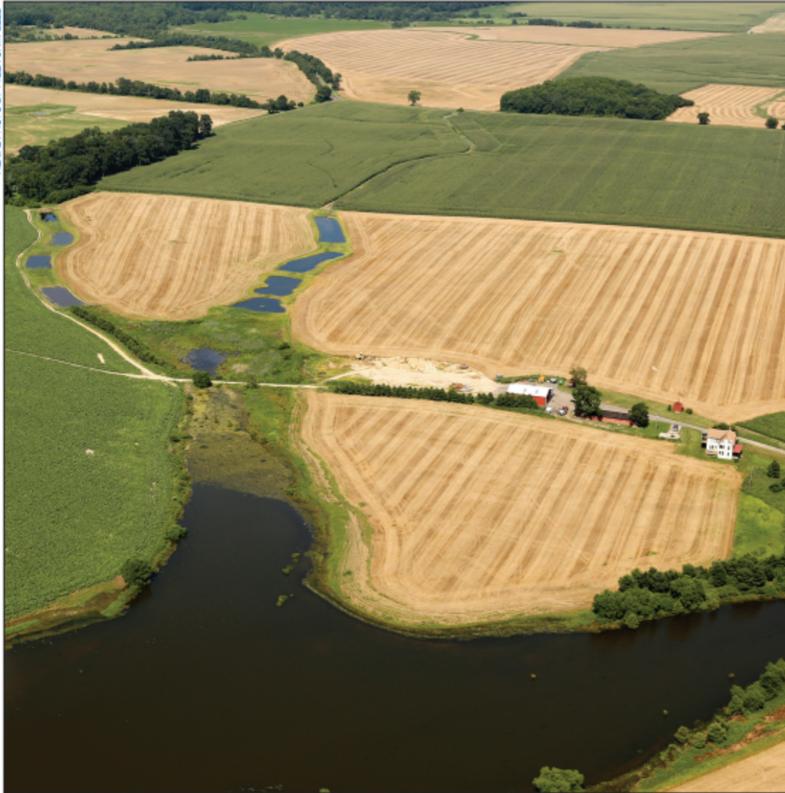
STORMWATER CATCHERS: Sam Owings redesigned his waterways with wetland cells to slow and absorb stormwater coming off uplands before trickling into the pond.
