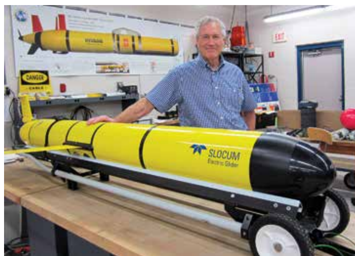
UMCES scientists adopt and implement the newest technologies, including the ocean glider instrument depicted here that autonomously surveys the ocean environment.
