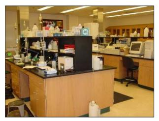
and major ions (by ion chromatography). The third water chemistry lab is used for the automated analysis of water samples for concentrations of metals by ICP-AES; acidity, alkalinity, and ANC by titration; nutrients, aluminum, and silica by flow injection analysis; and carbon species (DOC, TOC, DIC, TC) by the UV-assisted persulfate digestion technique.
