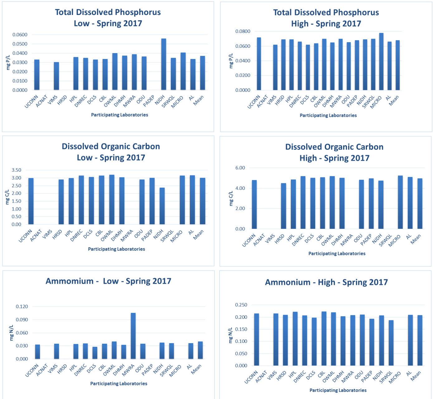
Figure 5. Total dissolved phosphorus; dissolved organic carbon, and ammonium. Spring 2017.
