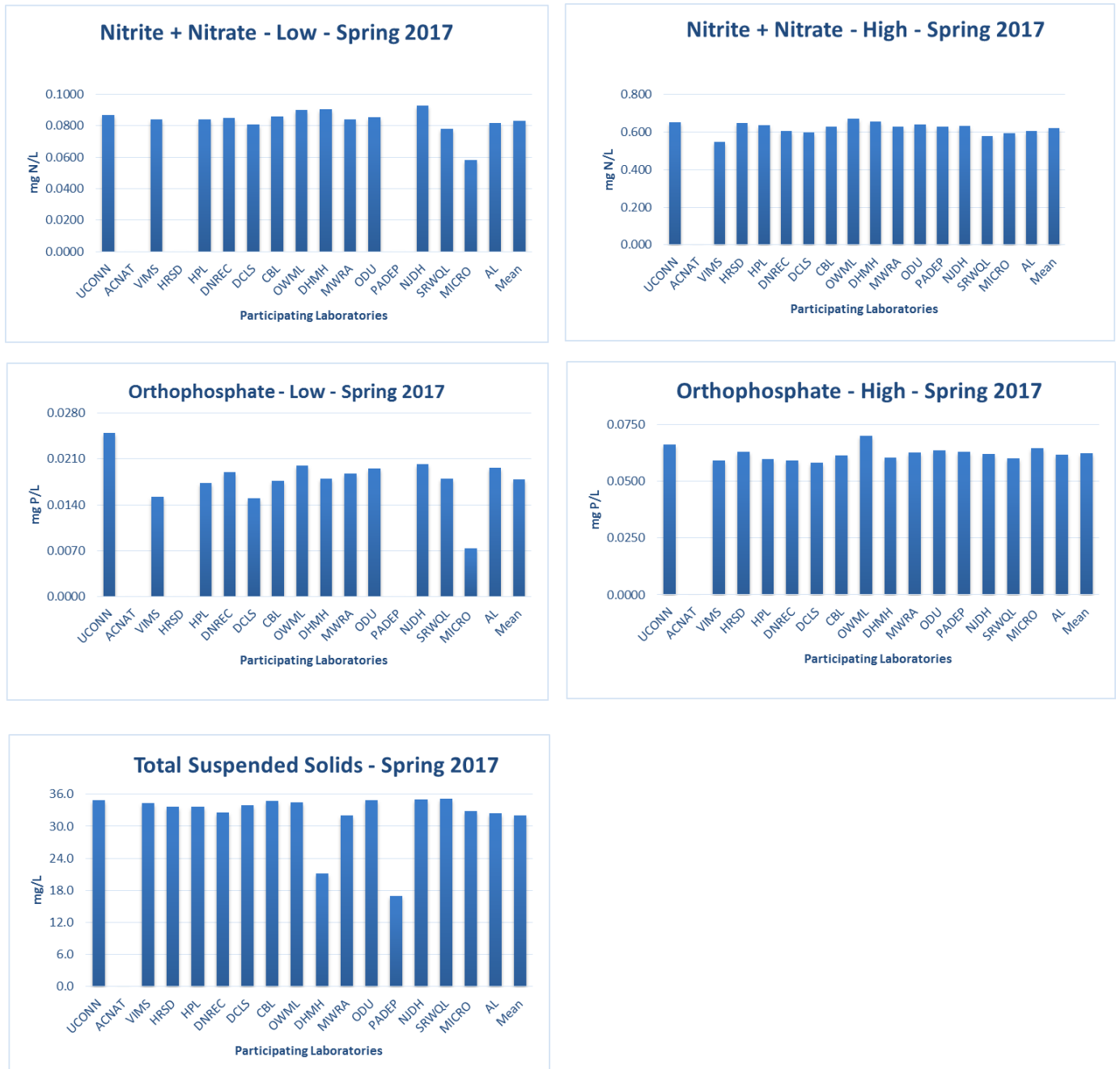
Figure 6. Nitrite plus nitrate, orthophosphate, and total suspended solids. Spring 2017.
