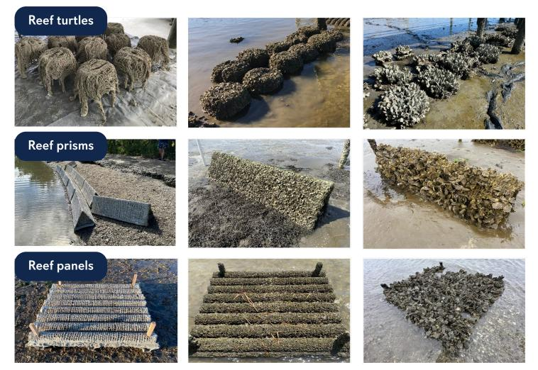
Jute Reinforced Calcium Sulfoaluminate (JR-CSA) in the shape of reef turtles (top), reef prisms (middle), and reef panels (bottom) upon deployment (left) and 6 months (middle) and 18 months (right) post-deployment. Photos courtesy of Mark Clark.
