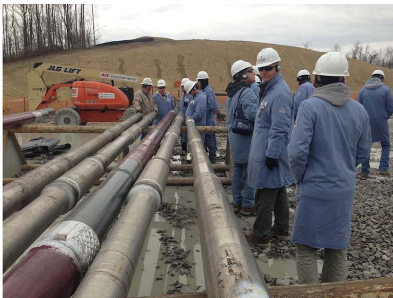
Figure 3-1: Horizontal drilling technology requires the ability to make a turn from vertical to horizontal drilling at depths ranging from 2,000 to 9,000 ft below the surface. These flexible drilling pipes are used to accomplish this task.
