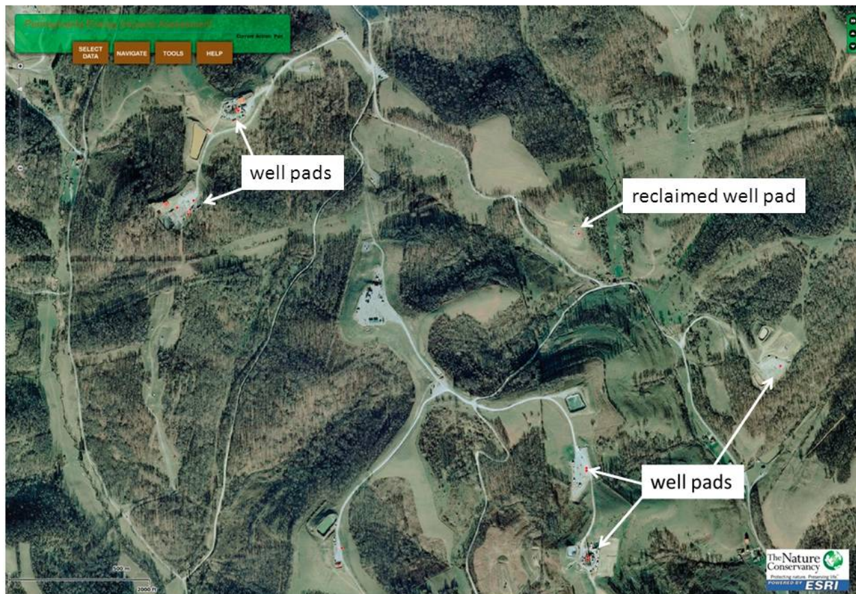
Figure 1-2. Air photo showing a densely-clustered well pad development in Pennsylvania. Drilled Marcellus gas wells are identified as red dots. Screen shot from web-based map viewer at http://maps.tnc.org/paenergy/ developed by The Nature Conservancy (website accessed February 8, 2013).
