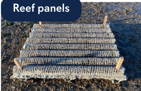
Jute Reinforced Calcium Sulfoaluminate (JR-CSA) in the shape of reef turtles (top), reef prisms (middle), and reef panels (bottom) upon deployment (left) and 6 months (middle) and 18 months (right) post-deployment. Photos courtesy of Mark Clark.
