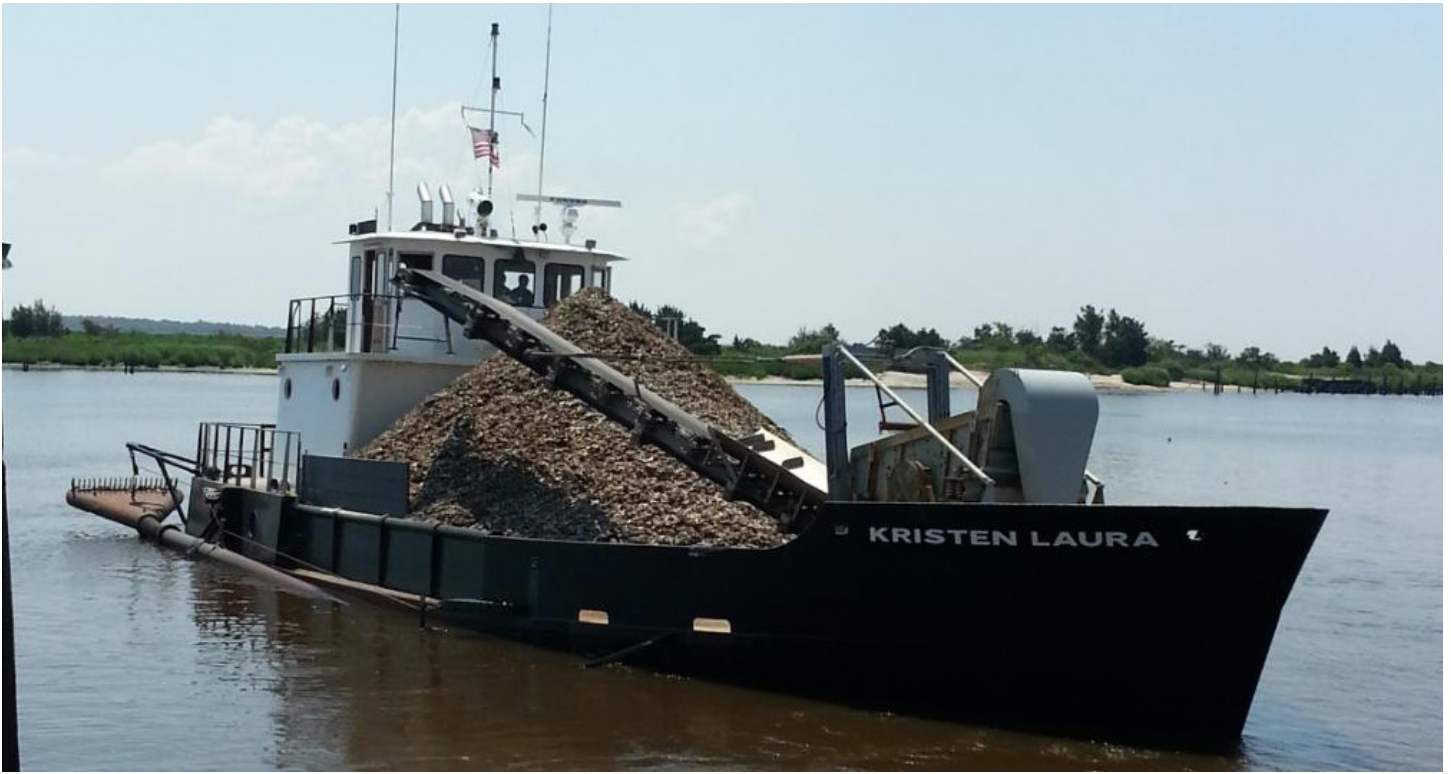
Suction dredge boat with a load of dredged shell in Delaware Bay. The head of the suction dredge is at the stern. Photo courtesy of Steve Fleetwood.
